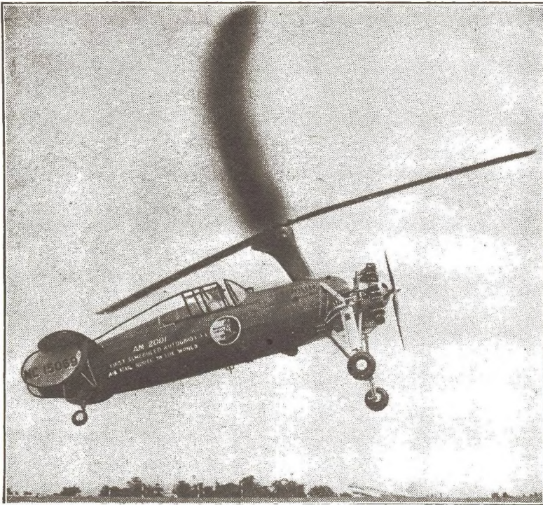
"First Scheduled Autogiro Air Mail Route in the World" are the words lettered on the fuselage of this Kellett KD1B. This job is a one-place craft, with an enclosed compartment. The high speed is 125 m.p.h.—and the low speed, from what we've heard, is 0 m.p.h. The plane plies daily from the Camden, N. J., Airport to the Philadelphia postoffice, where it sets down on the roof.
