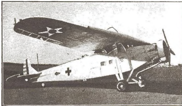
This Fokker C-15A is many years old, but the Air Corps still finds use for it as a flying ambulance. Originally designed as a cargo craft, the C-15A is powered with a 575-h.p. Cyclone. Every one is comfortable in this job during the cold winter—except the poor pilot. He has to sit in an open cockpit right behind the trailing edge of the full cantilever wing.
